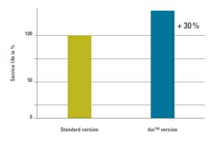
This benefit however can only be fully realized if the needle rotation system is adapted accordingly. If the rotation system is adjusted for this new material, the needles can remain in the board up to 30 % longer than with the standard material, and the product properties remain the same over a longer period of time.
