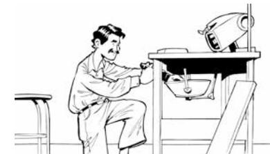
8. The mechanic searches for needle fragments in the sewing machine and in the oil bath.
