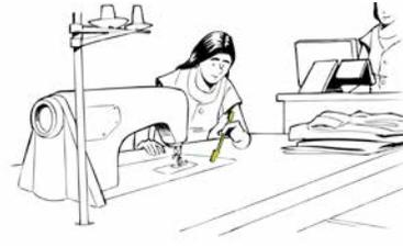
3. The operator searches the workstation with the magnetic tool.
