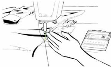
1. The operator removes the mounting shank of the needle from the sewing machine and the broken needle piece hanging from the thread.
