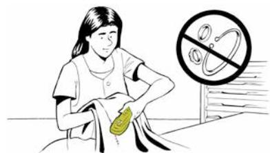
6. The operator uses the hand-held scanner to search first at the point most recently sewn, and then over the entire garment.
